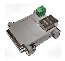
**CNC PodAn** Ethernet controller with two LPT outputs. Various inexpensive breakout boards can be connected to it. Also integrated complete power amplifiers, like the Triple-Beast. There are extensions to be able to use the 2nd LPT board and also an extension for plasma cutting THC-Control. Works with all software variants.
