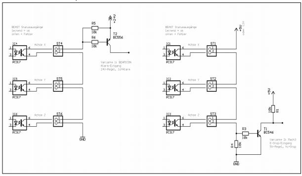
The figure above shows two circuit examples, one for 24V level (e.g. PLC systems) and one for 5V level (PC parallel port, Mach3 without breakout board or from another manufacturer). The status outputs of the BEAST output stages are connected in series. A fault in at least one output stage, the interruption of a cable or a power failure will certainly lead to an alarm message to the control system.
